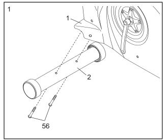
2. Attach the Rear Stabilizer (3) to the Frame (1) with two M10 x 85mm Button Screws (56).
